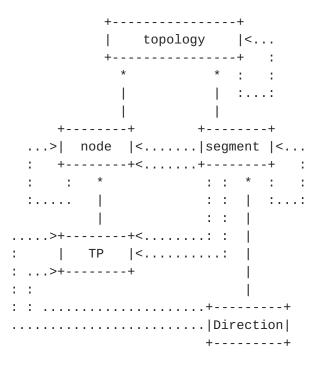
The basic information model works as follows: A service topology contains service nodes and segments. A segment connects two nodes (a source and a destination) and have direction, may be unidirectional or bidirectional. unidirectional is one where traffic is passed through a set of SF nodes in one forwarding direction only. Bidirectional is one where traffic is passed through a set of SF nodes in both
