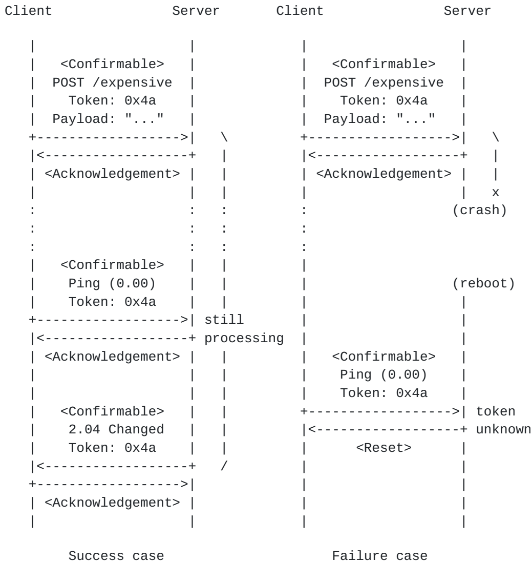
Figure 1: Liveliness check of a request with token 0x4a
