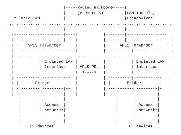
Figure 2: PE Reference model
