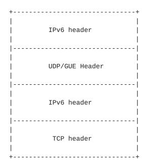
The addresses in the outer IPv6 header indicate the physical nodes (source and destination NVEs) in the network. The inner IPv6 addresses are IPv6 addresses within the virtual network specified by the VNID in the GUE header.
