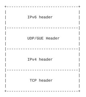
The addresses in the outer IPv6 header indicate the physical nodes (source and destination NVEs) in the network. The inner IPv4 addresses are in the virtual network specified by the VNID in the GUE header.
