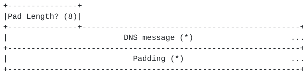
Figure 1: DNS frame format
