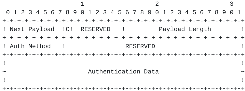
Figure 14: Authentication Payload Format
