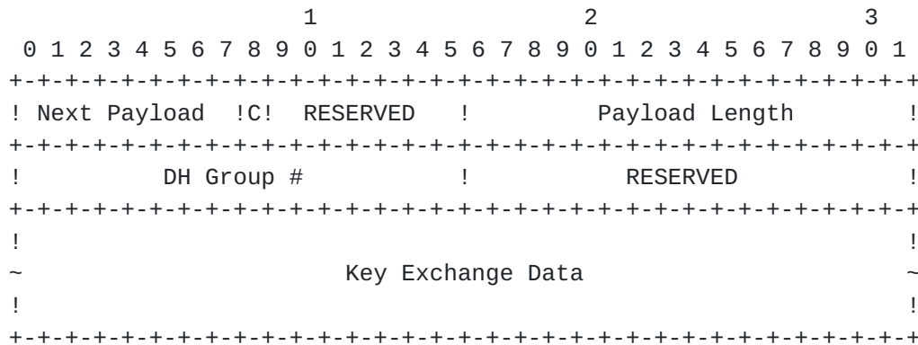
Figure 10: Key Exchange Payload Format
