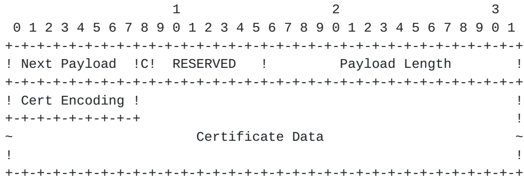
Figure 12: Certificate Payload Format
