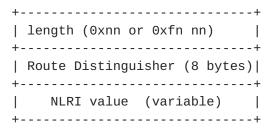
Figure 2: Flow-spec NLRI for MPLS
