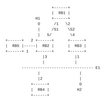
Based on the topology, a distribution tree rooted at RB1 can be calculated by each RBridge, which is given in Figure 2, where the node represented by a triangle is the pseudonode for E1. H1 and H2 are not RBridges, so they are not on this tree.
