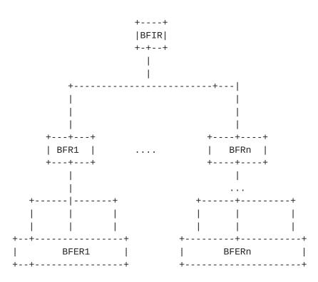
BRF1 and BFRn, and other BFRs in between, can share one bit because they are receiving all the content and don't need pruning. From BFR1 to BFER1, there are 3 ways to reach BFER1. So these 3 ways can be assigned with different bits. But these 3 bits can be reused in the group from BFRn to BFERn, and other groups in between, which share the same topology as the group from BFR1 to BFER1.
