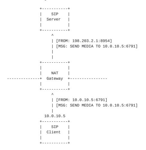
The purpose of STUN [STUN] is to allow clients to detect this situation and determine the address mapping. They can then place the appropriate address in their application-level messages. This is done by making use of an external STUN server. That server is able to determine the translated address and tell the STUN client, as shown below.
