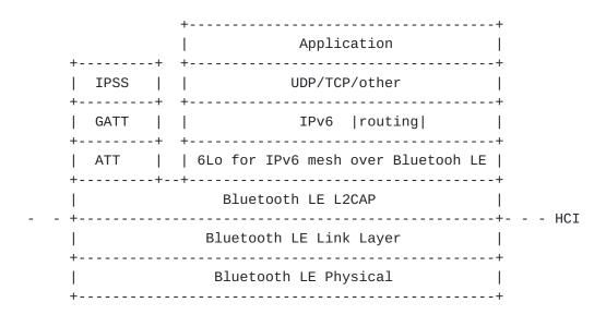
Figure 1: Protocol stack for IPv6 mesh over Bluetooth LE links.
