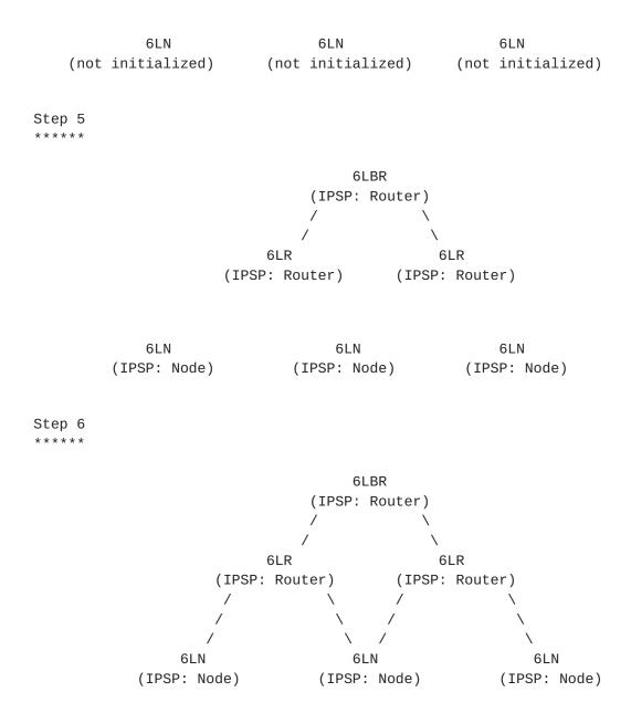
Figure 3: An example of connection establishment and use of IPSP roles in an IPv6 mesh over Bluetooth LE links.
