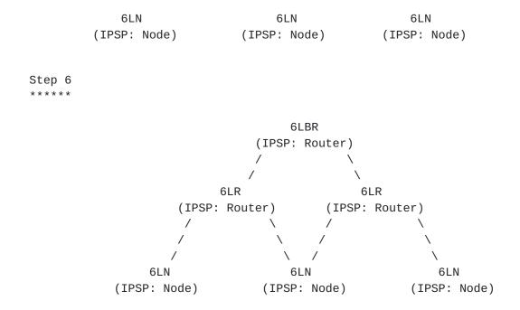
Figure 3: An example of connection establishment and use of IPSP roles in an IPv6 mesh over Bluetooth LE links.
