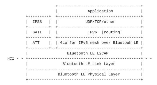
Figure 1: Protocol stack for IPv6 mesh over Bluetooth LE links.
