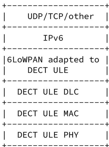
Figure 3: IPv6 over DECT ULE Stack
