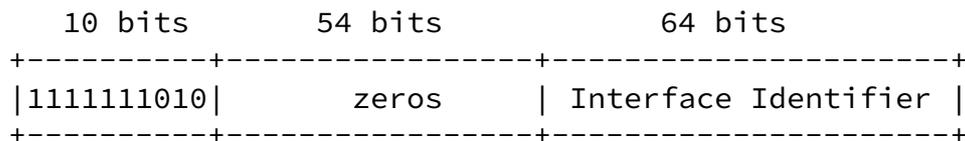
Figure 4: IPv6 link-local address in DECT ULE
