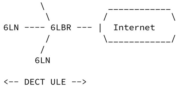
Figure 5: DECT ULE network connected to the Internet
