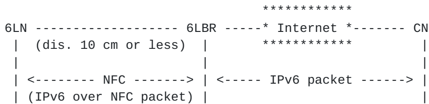
Figure 8: NFC-enabled device network connected to the Internet
