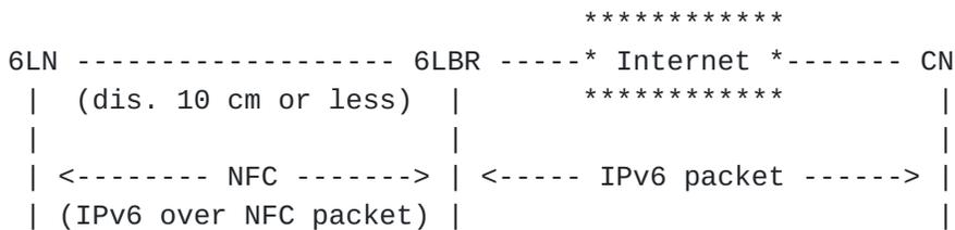
Figure 13: NFC-enabled device network connected to the Internet
