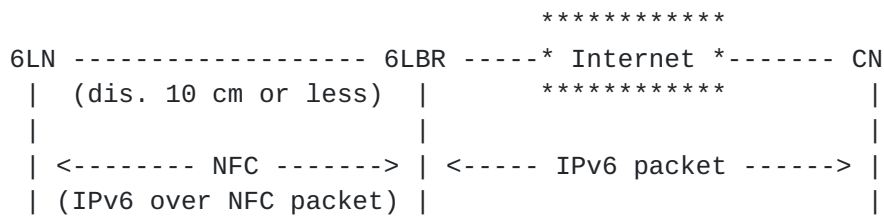
Figure 10: NFC-enabled device network connected to the Internet
