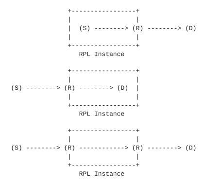
In the scenarios above, R may indicate a RPL Border Router (when connecting to other routing domains) or a RPL Router (when connecting
