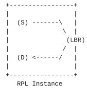
In the above scenario, datagrams travel from S to D through LBR. Between S and LBR, the datagrams are routed using the DAG built by RPL and do not contain a SRH. LBR encapsulates received datagrams unmodified using IPv6-in-IPv6 and the SRH is included in the outer IPv6 header.
