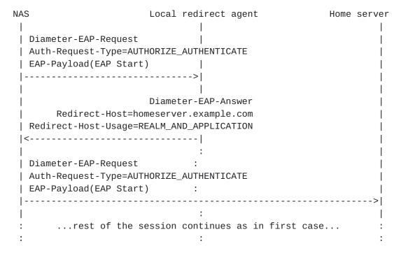
The advantage of this scenario is that knowledge of realms and home servers is centralized to a redirect agent, and it is not necessary to modify the NAS configuration when, e.g., a new roaming agreement is done.
