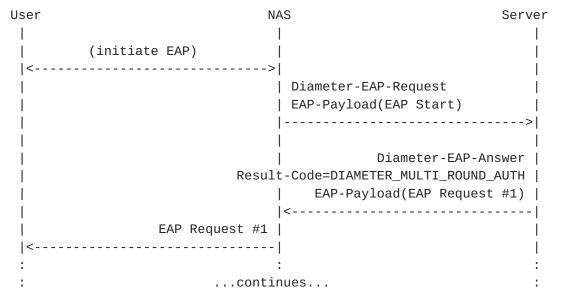
The initial Diameter-EAP-Answer in a multi-round exchange normally includes an EAP-Request/Identity, requesting the EAP client to identify itself. Upon receipt of the EAP client's EAP-Response, the access device will then issue a second Diameter-EAP-Request message, with the client's EAP payload encapsulated within the EAP-Payload AVP.
