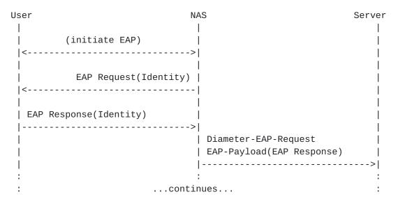
The conversation continues until the Diameter server sends a Diameter-EAP-Answer with a Result-Code AVP indicating success or failure, and an optional EAP-Payload. The Result-Code AVP is used by the access device to determine whether service is to be provided to the EAP client. The access device MUST NOT rely on the contents of the optional EAP-Payload to determine whether service is to be provided.
