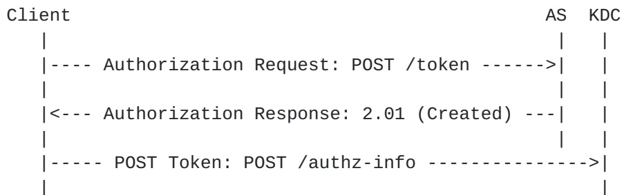
Figure 3: Message Flow of Join Authorization
