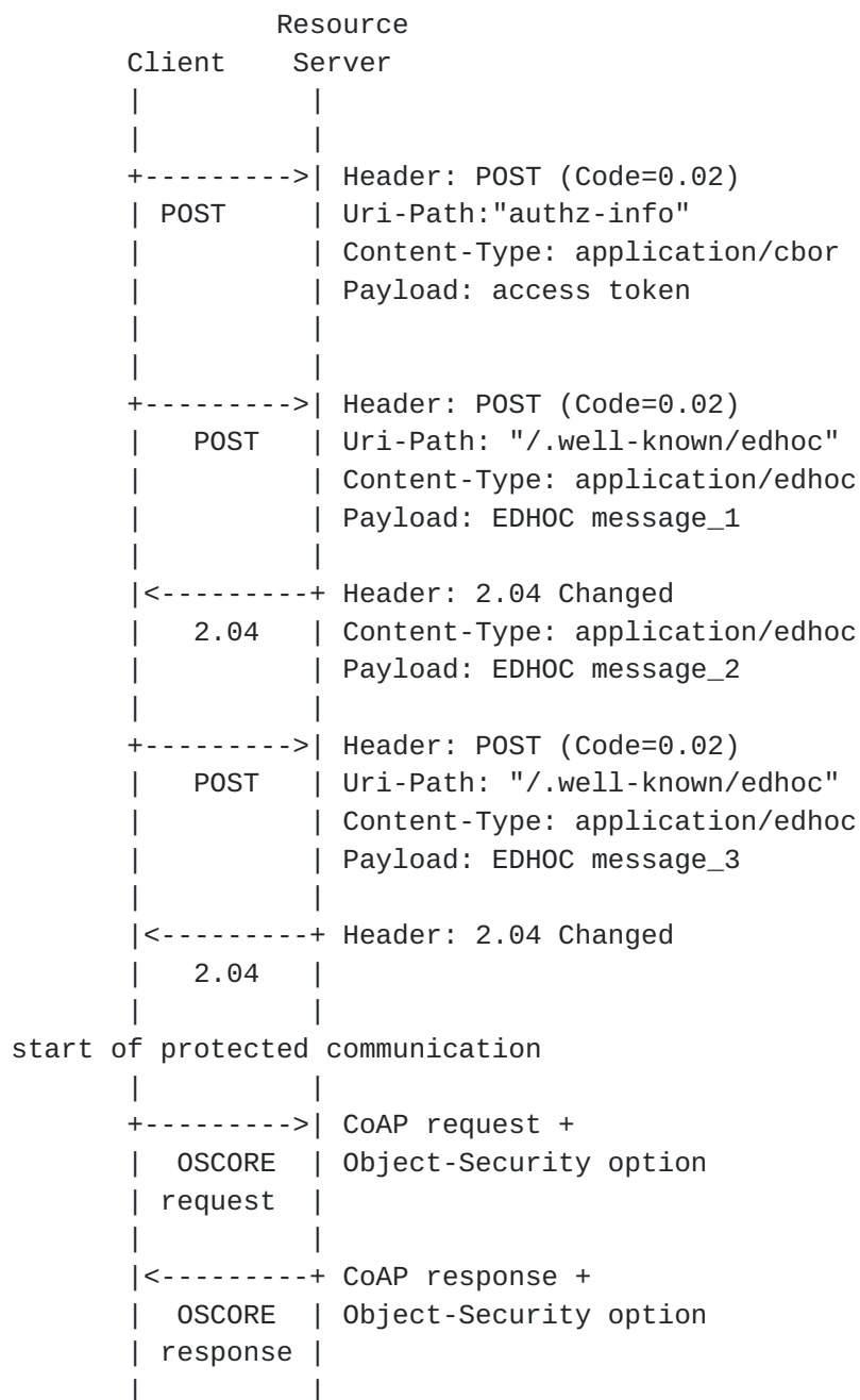
Figure 7: Access token and key establishment with EDHOC
