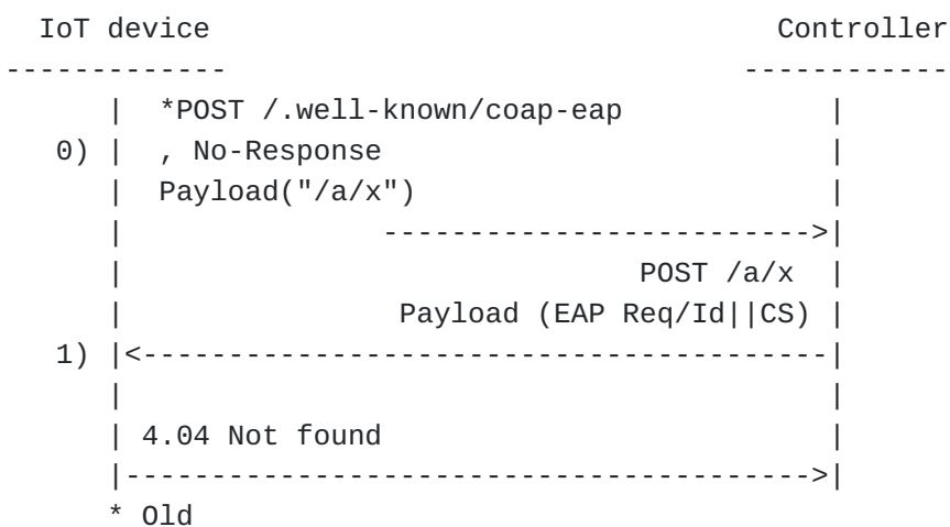
Figure 5: /.well-known/coap-eap with no ongoing authentication from the EAP authenticator
