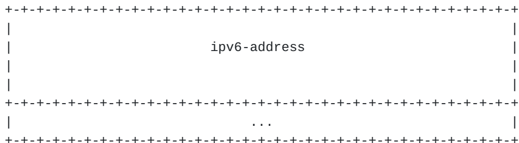
Figure 2: Format of the IPv6 Addresses Field
