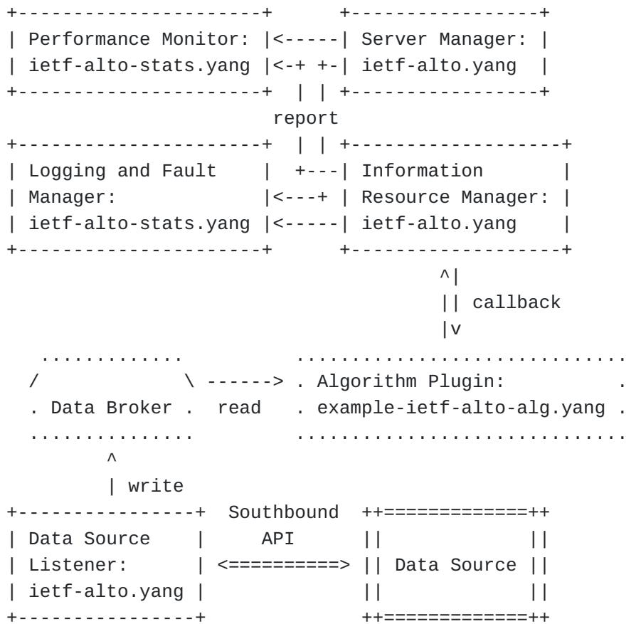
Figure 1: A Reference ALTO Server Architecture and YANG Modules
