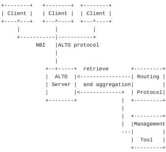
Figure 1.End to End Path Cost Metrics Exposing
