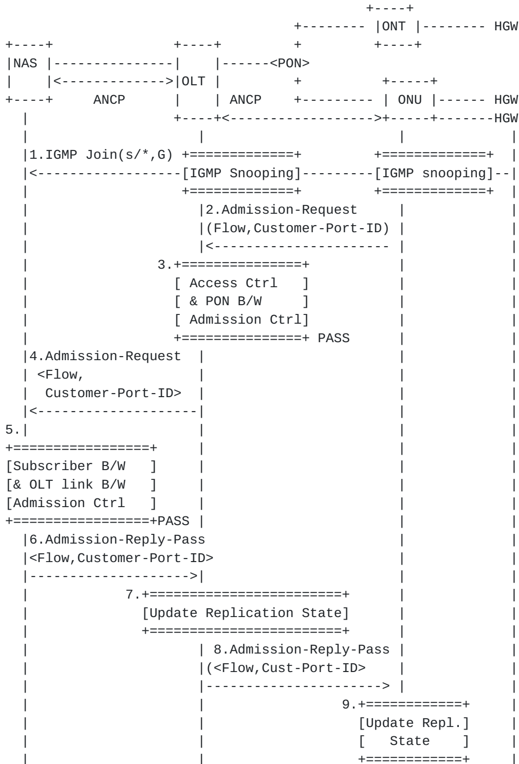
Figure 9: Interaction between NAS & ANX for Multicast Bandwidth Admission Control in the All-ANCP ANX control model upon success. Similar functionality will be required when OMCI is enabled between the OLT and ONT/ONU in the ANCP+OMCI ANX control model. In this latter case, the OLT will act as ANCP-OMCI gateway.
