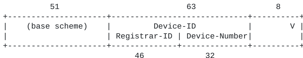
Figure 4: ACP V8 Addressing Sub-Scheme
