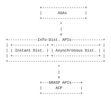
As the Fig 1 shows, the information distribution module two submodules for instant and asynchronous information distributions, respectively, and provides APIs to ASAs. Specific Behaviors of modules are described in Section 5.
