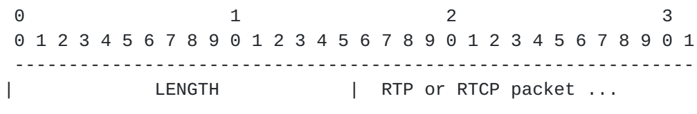
Figure 1 -- The bitfield definition of the framing method.
