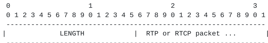
Figure 1 -- The bitfield definition of the framing method.
