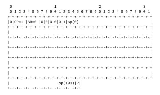
In the payload the speech frame is not damaged at the IP origin (E=1), the coding rate is 9.7 kbps(CR=1), the base rate is 7.8 kbps (BR=0), and the DTX mode is off. There is no byte alignment (A=0) and no redundancy (R=0). The encoded speech bits - s(0) to s(193) - are placed immediately after TOC. Finally, one zero bit is added at the end as padding to make the payload byte aligned.
