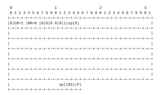
In the payload the speech frame is not damaged at the IP origin (E=1), the coding rate is 9.7 kbps(CR=1), the base rate is 7.8 kbps (BR=0), and the DTX mode is off. There is no byte alignment (A=0) and no redundancy (R=0). The encoded speech bits - s(0) to s(193) - are placed immediately after TOC. Finally, one zero bit is added at the end as padding to make the payload byte aligned.
