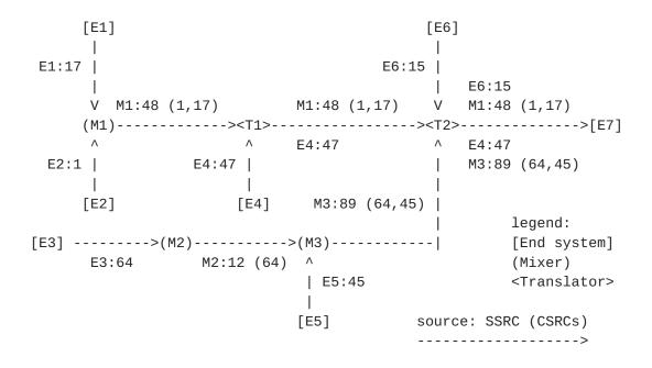
Figure 3: Sample RTP network with end systems, mixers and translators
