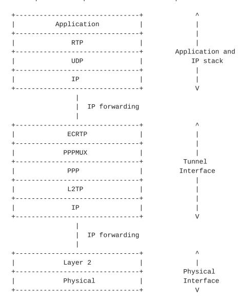
A protocol stack is configured to create an L2TP tunnel interface to a destination host. The tunnel is configured to negotiate the PPP connection (using NCP IPCP) with ECRTP header compression and PPPMUX. IP forwarding is configured to route RTP packets to this tunnel. The destination UDP port number could distinguish RTP packets from non- RTP packets.
