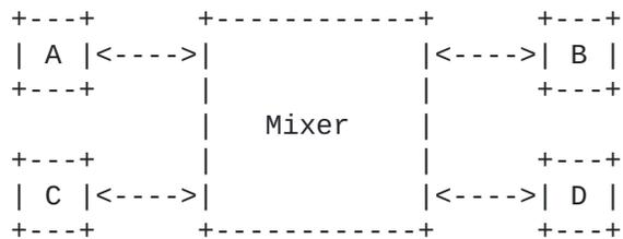
Figure 14: RTP Mixer with Only Unicast Paths
