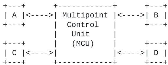
Figure 19: Point to Multipoint Using Content Modifying MCUs
