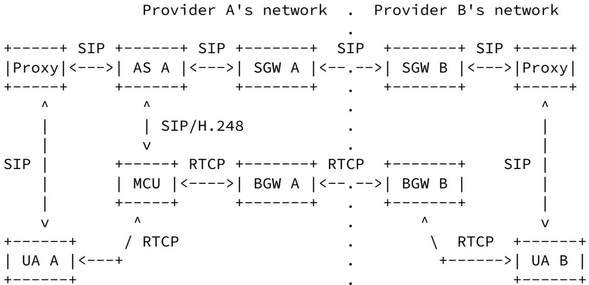
Figure 4: Comparison Signaling Topology
