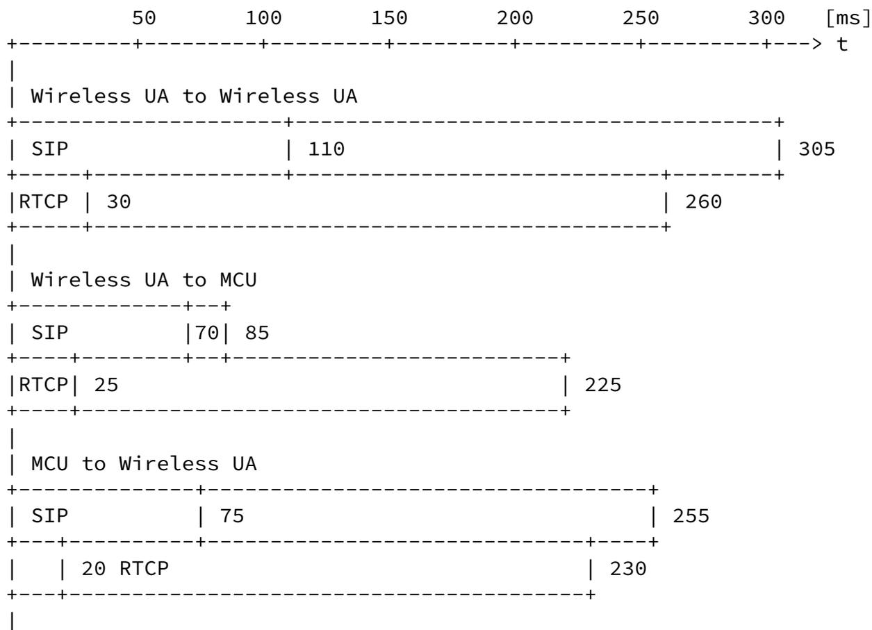
Figure 6: Mobile Access Transmission Delay Comparison
