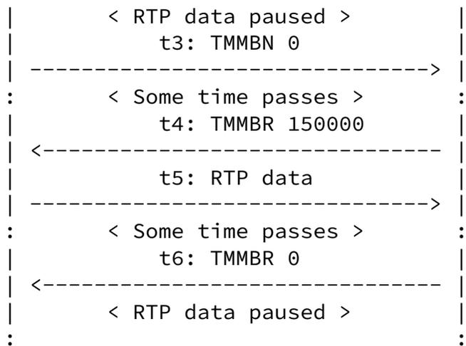
Figure 14: TMMBR Pause and Resume in Point-to-Point
