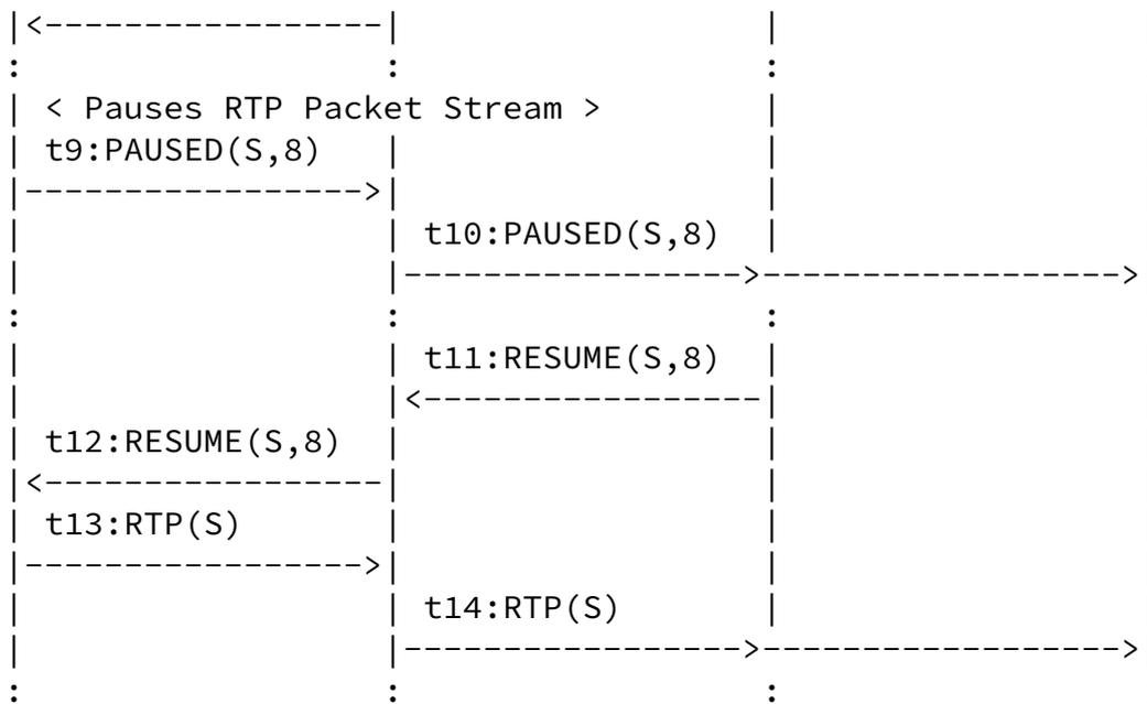
Figure 19: Pause and Resume Operation Between One Sender and Two Receivers Through Translator
