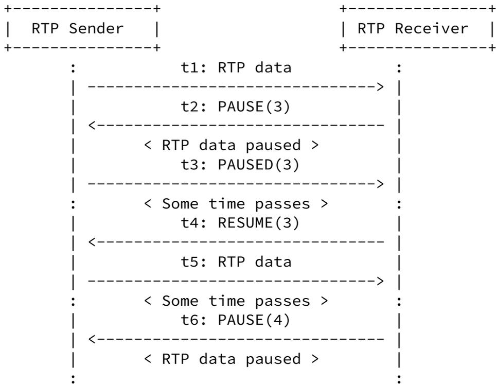
Figure 13: Pause and Resume Operation in Point-to-Point
