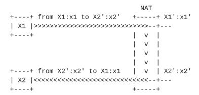
Hairpinning allows two endpoints on the internal side of the NAT to communicate even if they only use each other's external IP addresses and ports.
