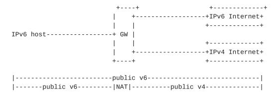
The proposed NAT64/DNS64 is perfectly suitable for this particular scenario. The deployment of the NAT64/DNS64 would be as follows: The NAT64 function should be located in the GW device that connects the IPv6 site to the IPv4 Internet. The DNS64 functionality can be placed either in the local recursive DNS server or in the local resolver in the hosts.
