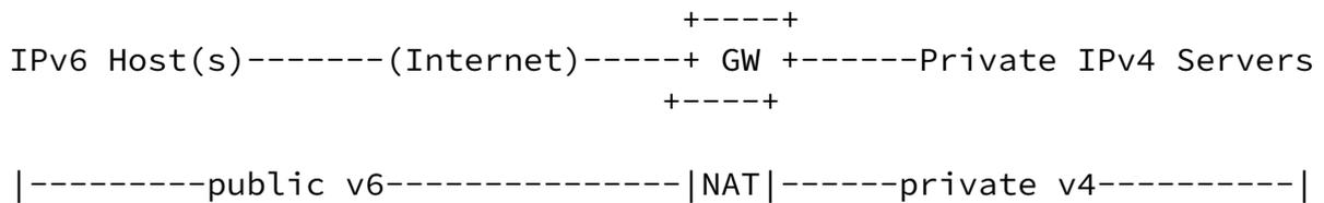
This scenario can again be perfectly served by the NAT64 approach. In this case the NAT64 functionality is placed in the GW device connecting the IPv6 Internet to the server's site. In this case, the DNS64 functionality is not required in general since real (i.e. non synthetic) AAAA RRs for the IPv4 servers containing the IPv6 representation of the IPv4 address of the servers can be created. See more discussion about this in [[I-D.ietf-behave-dns64](#)]
