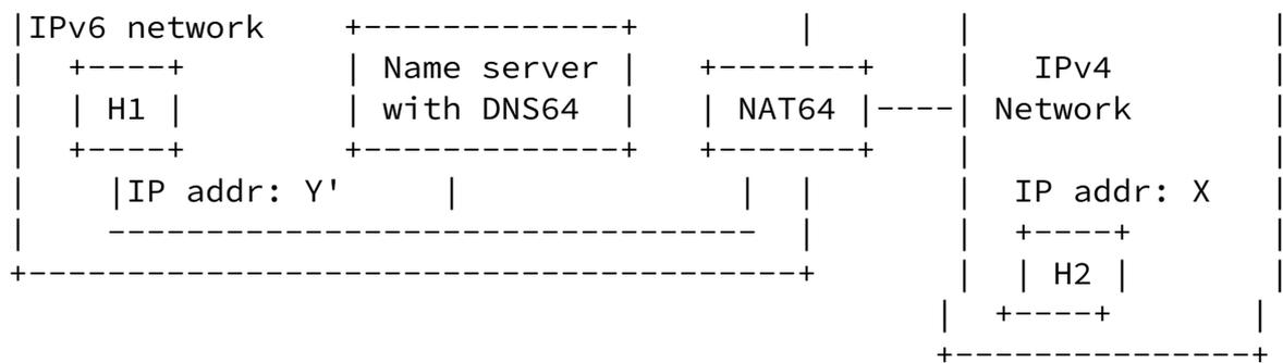
The figure shows a IPv6 node H1 which has an IPv6 address Y' and an IPv4 node H2 with IPv4 address X.
