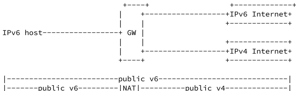
The proposed NAT64/DNS64 is perfectly suitable for this particular scenario. The deployment of the NAT64/DNS64 would be as follows: The NAT64 function should be located in the GW device that connects the IPv6 site to the IPv4 Internet. The DNS64 functionality can be placed either in the local recursive DNS server or in the local resolver in the hosts.
