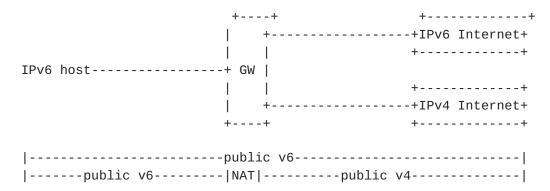
The proposed NAT64/DNS64 is perfectly suitable for this particular scenario. The deployment of the NAT64/DNS64 would be as follows: The
