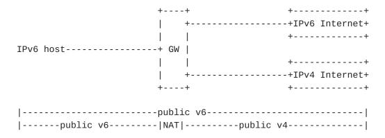
The proposed NAT64/DNS64 is perfectly suitable for this particular scenario. The deployment of the NAT64/DNS64 would be as follows: The NAT64 function should be located in the GW device that connects the IPv6 site to the IPv4 Internet. The DNS64 functionality can be placed either in the local recursive DNS server or in the local resolver in the hosts.
