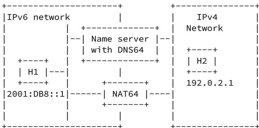
The figure above shows an IPv6 node H1 with an IPv6 address 2001:DB8::1 and an IPv4 node H2 with IPv4 address 192.0.2.1 H2 has h2.example.com as FQDN.
