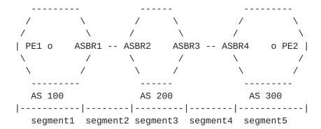
The inter-as segmentation procedures specified so far (RFC 6513/6514, 7117, and <u>Section 5</u> of this document) requires all ASBRs to be involved, and Ingress Replication is used between two ASBRs in different ASes.
