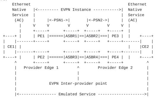
iBGP sessions are established between PE1, PE2, ASBR1 and ASBR3, possibly via a BGP route-reflector. Similarly, iBGP sessions are established between PE3, PE4, ASBR2 and ASBR4. eBGP sessions are established among ASBR1, ASBR2, ASBR3, and ASBR4.
