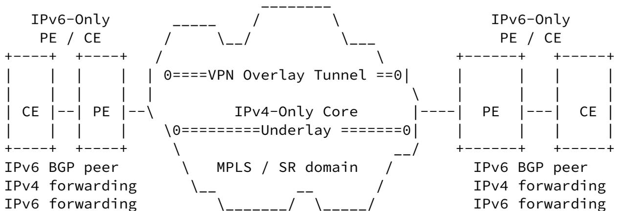
Figure 8: Test-2 E2E IPv6-Only PE-CE, VPN over IPv4-Only Core
