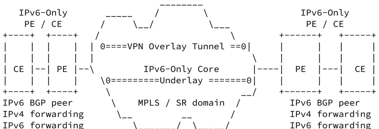
Figure 10: Test-4 E2E IPv6-Only PE-CE, VPN over IPv6-Only Core
