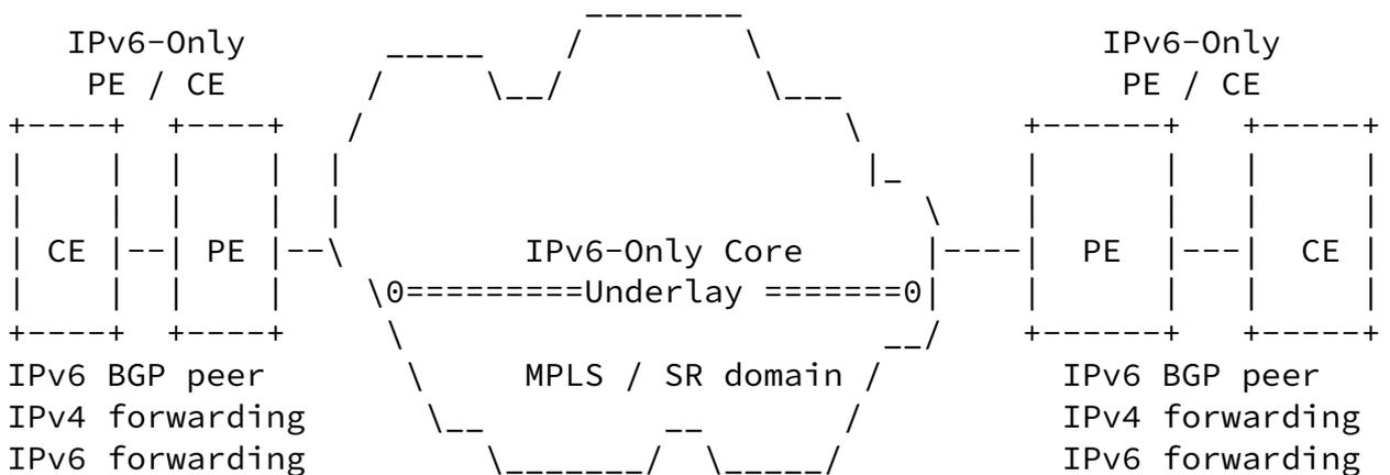
Figure 9: Test-3 E2E IPv6-Only PE-CE, Global Table over IPv6-Only Core (4PE)
