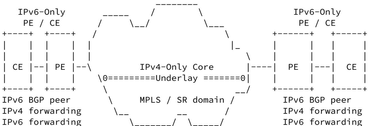
Figure 7: Test-1 E2E IPv6-Only PE-CE, Global Table over IPv4-Only Core (6PE)
