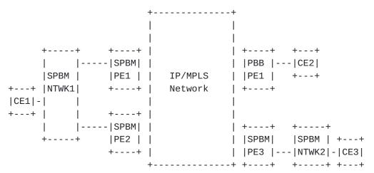
Figure 1: PBB and SPBM EVPN Network
