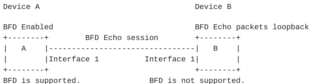
Figure 1: Unaffiliated BFD Echo diagram
