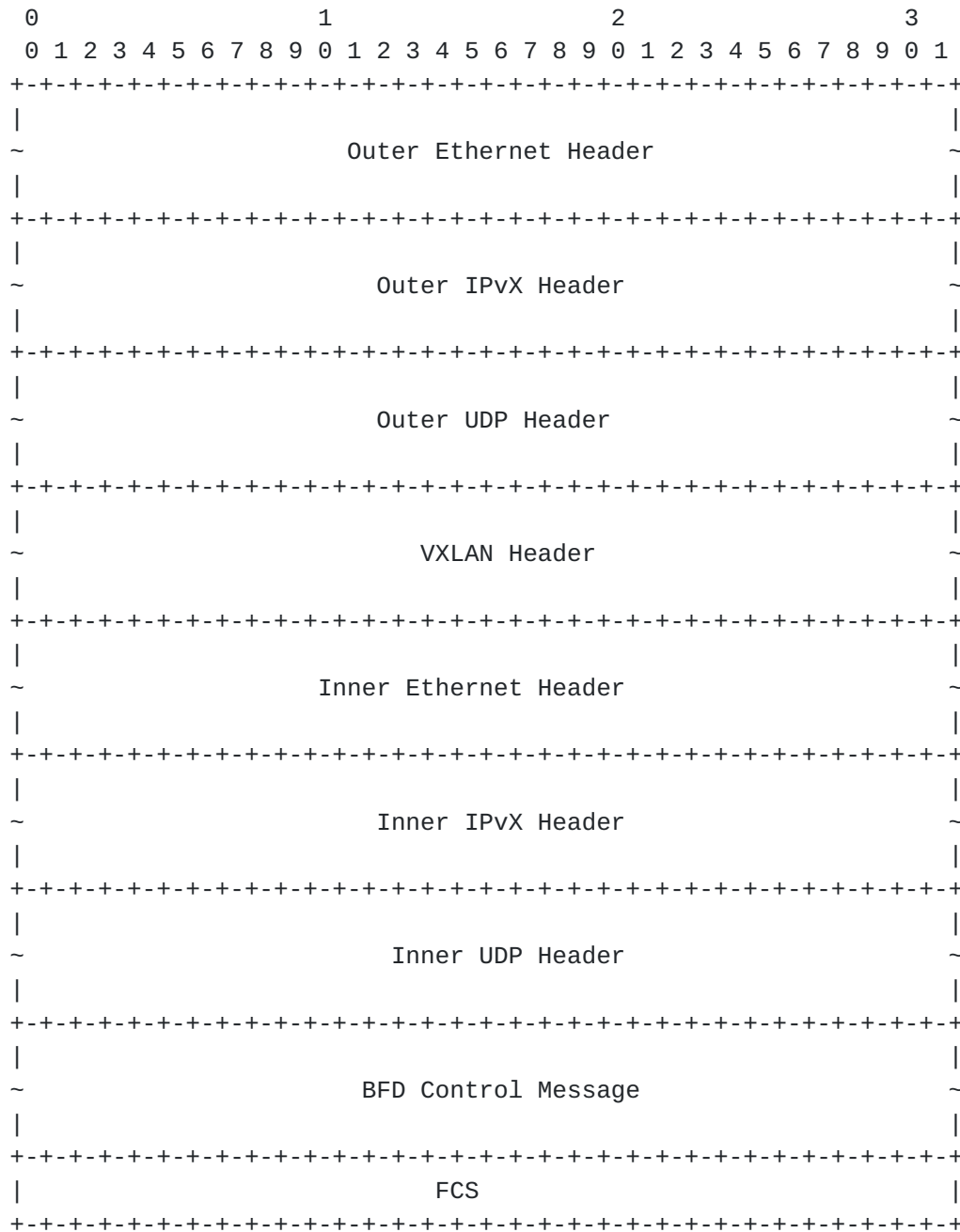
Figure 2: VXLAN Encapsulation of BFD Control Message
