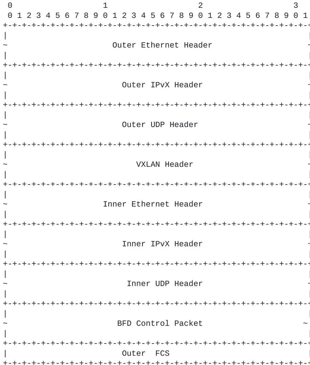
Figure 2: VXLAN Encapsulation of BFD Control Packet
