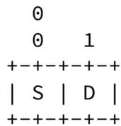
Figure 1: OAM field of BIER Header format
