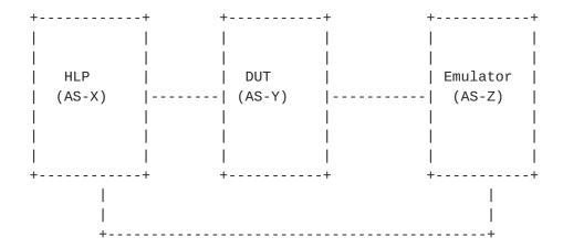
Figure 2 Three Node Setup for eBGP and iBGP Convergence
