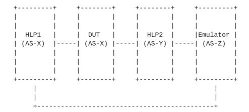
Figure 4 Four Node Setup for EBGP and IBGP Convergence
